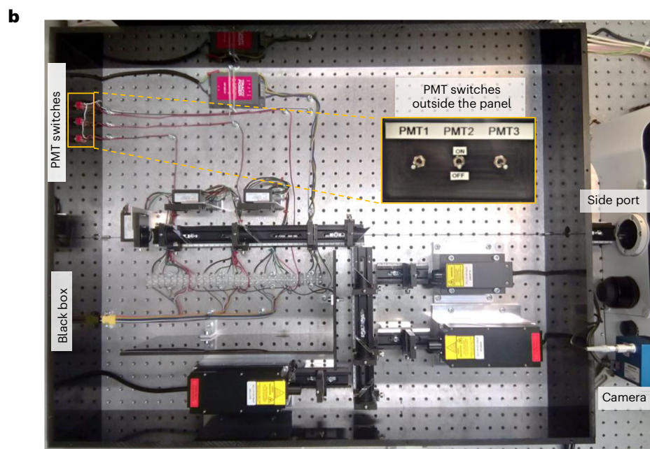
Fig. 5 | Breadboard layout. a , Map depicting the positions of the assembly components to be fixed on the breadboard at their respective coordinates. The black box (thick gray rectangle) defines the periphery of the assembly. The coordinate system has the origin at the left-bottom thread on the periphery and a single unit in the layout is equal to the distance between two holes (2.5 cm). As an example, the coordinates for the screw positions of support blocks for rail E and laser L1 are shown in red and detailed positioning is presented in Extended Data Fig. 2. The line M–M' represents the plane of the microscope's left side port that should make a 90° angle with rail D. b , Image of the finished assembly with every component corresponding to the map.
